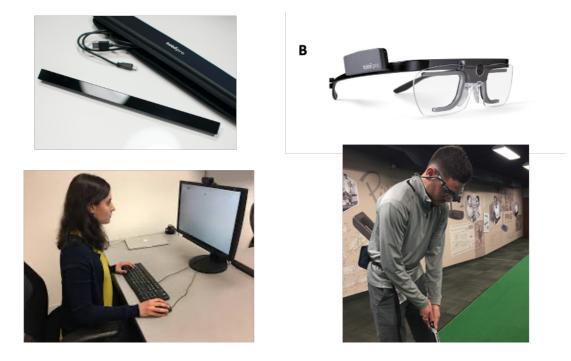
**Figure 2.** Images of the fixed (left) and wearable (right) eye trackers used in the School of Psychology. The eye tracker in panel A is the Tobii X3 120. In the lower panel, the X3 120 is attached to the bottom of the computer monitor as a participant performs a task. Panel B depicts the Tobii Glasses 2; in the lower panel, a participant wears the glasses while practicing golf.
